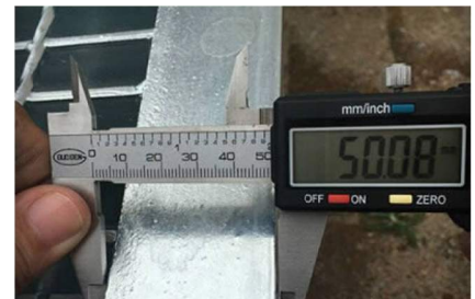
Angle bar size inspection
