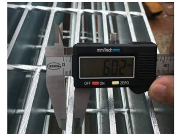
Bearing bar size inspection
